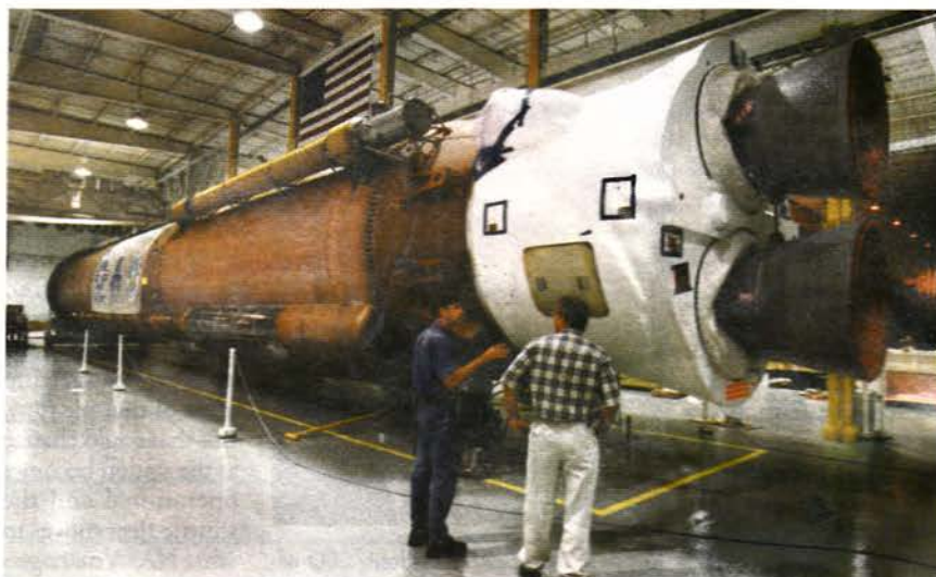
Lockheed Martin Atlas V EELV first stage undergoes final processing in Cape Canaveral's Atlas Spaceflight Operations Center. Russian RD-180 engine has twin nozzles.
