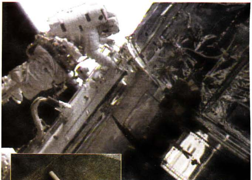
Astronaut John Grunsfeld positions the radiator for a new cryocooler on the aft shroud of the Hubble Space Telescope. Tiny turbines (inset) in the mechanical system carry heat away from the telescope's infrared camera.
