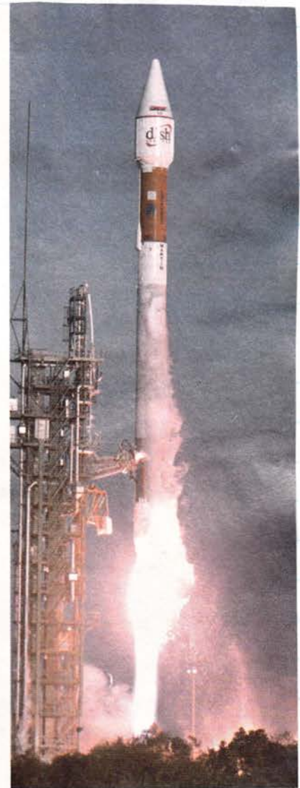
Lockheed Martin Atlas IIIB with a twin-engine stretched Centaur upper stage lifts off with 616,000-lb. thrust from its Russian RD-180 engine.
