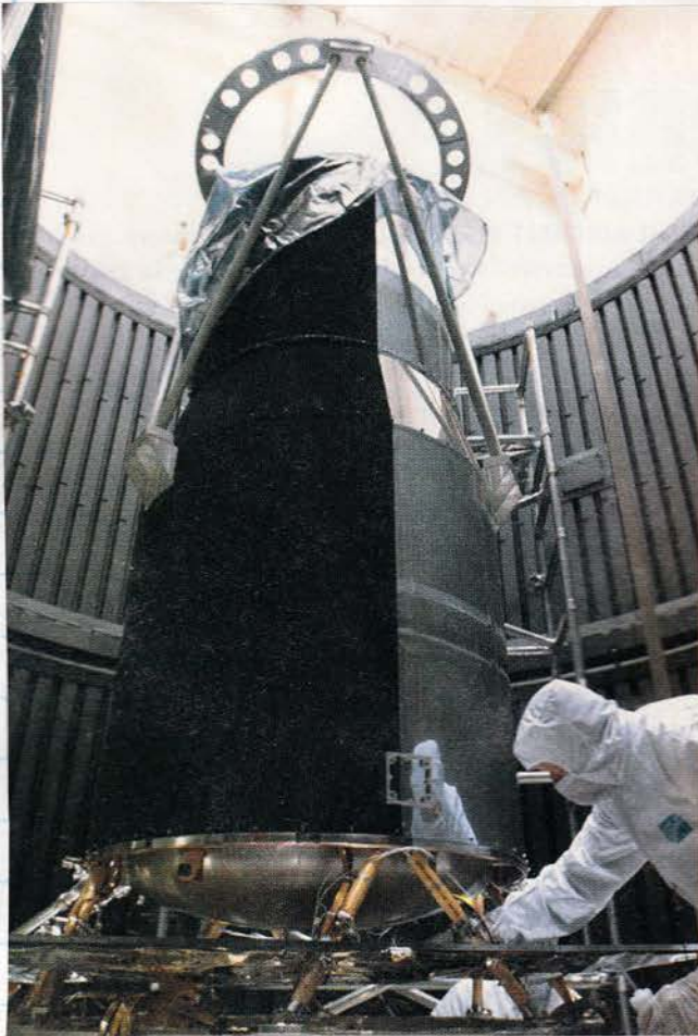
The heart of SIRTf is a Cryogenic Telescope Assembly, shown in a Ball Aerospace & Technologies test chamber. Low-conductivity struts thermally isolate the CTA from the spacecraft.
